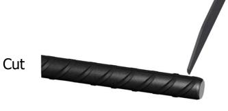
The rough cropped end of the reinforcing bar is removed to produce a clean square cut face.
