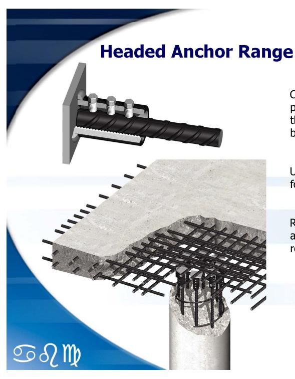
Comprises half an MBT coupler with a plate welded to one end which carries the full tension load of the bar when bearing against the concrete.
