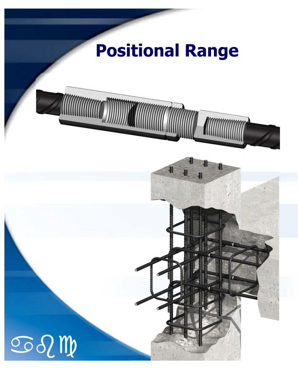
The two opposing bar ends are threaded with right hand tapered threads but are joined together using a three part positional coupler.
