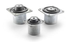
The AMC-MECANOCAUCHO HYDRAULIC CONE MOUNT is a combination of a spring component and a hydraulic shock absorber in the shape of a cone. With this both components can be tuned to each other. For good vibration insulation you need a low dampening coefficient but for movement control you need a high dampening coefficient. The AMC MECANOCAUCHO HYDRAULIC CONE MOUNTS combine these two completely different requirements in one single bearing.
