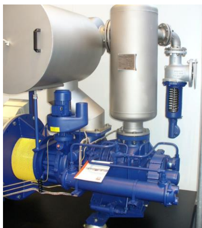
Figure 6.2.5.3-1: LESER Safety Valves in the non-upright position
