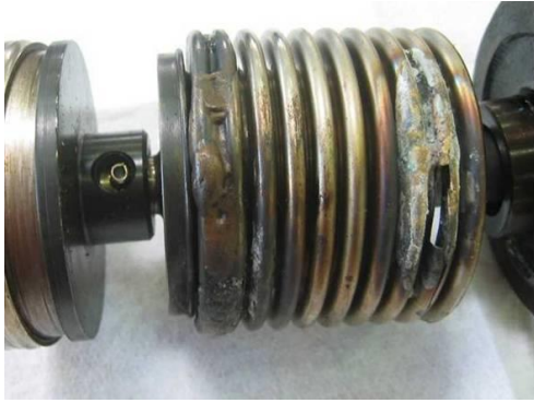
Figure 17.3.5-1: Symptom 16 - Corroded stainless steel bellows
