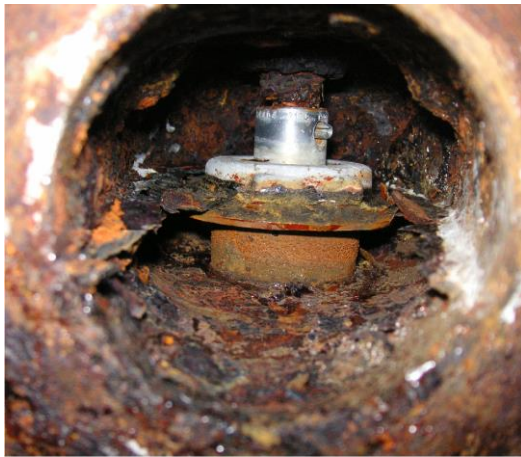
Figure 17.3.4-1: Symptom 12 - Strong corrosion in a safety valve
