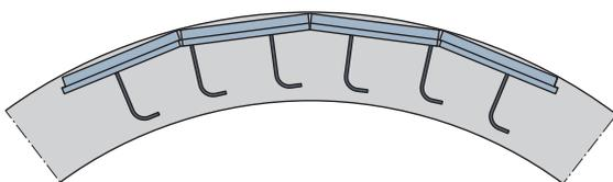
**HBT Element fitted to an convex curvature**
