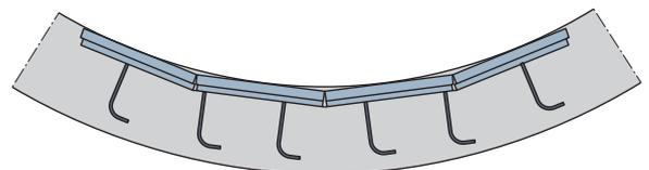
**HBT Element fitted to an concave curvature**
