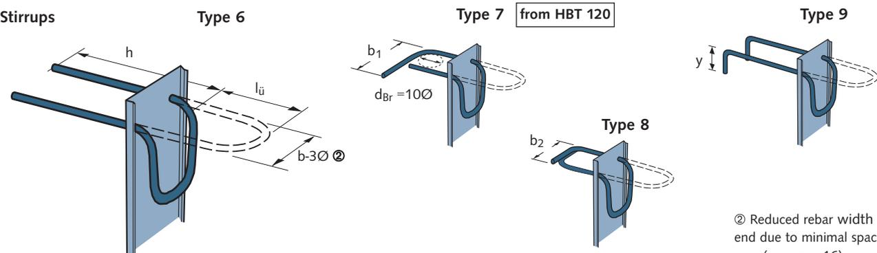
② Reduced rebar width at stirrup end due to minimal space in the case (see page 16)
