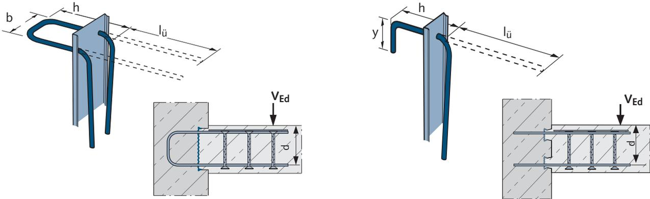
Please refer to the HDB Product information and approvals no. Z-15.1-249 and Z-15.1-270 when determining the shear reinforcement using HALFEN HDB-S Shear reinforcement.
