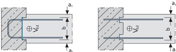
If the spaces between the HBT Cases are additionally subjected to shear load, then these must be designed as rough or suitably indented in accordance with DIN EN 1992-1-1. The edge areas can also be assumed as load bearing if  $a_1 \geq 50$  mm.
