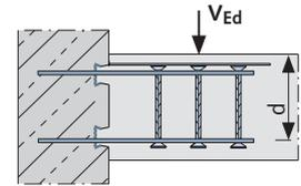
$$V_{Ed} \leq V_{Rd} \leq 0.3 \cdot V_{Rd,max}$$
