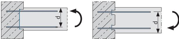
Tension zones: upper and lower component edges
