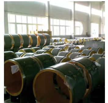
Preassembled cryogenic pipe supports
