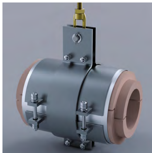
Special articulated cryogenic horizontal hanger support with clamping mechanism.
