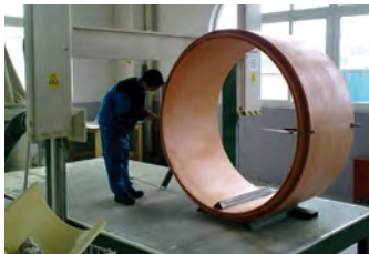
Special design for pipe diameter 1625,6mm
