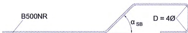
c) Execution with stainless reinforcing steel B500 NR, upper leg of shear bar carried out as loop
