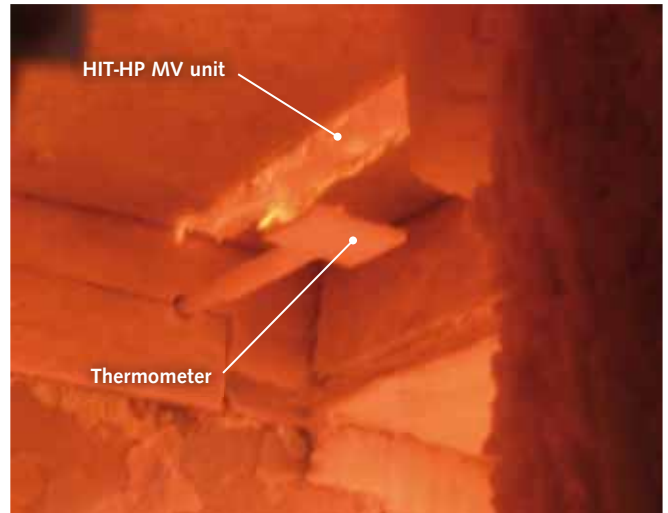
View into the fire test chamber during the HIT-HP MV fire-test after 120 minutes of exposure
