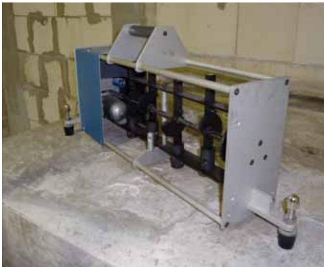
Standardised tapping machine according to EN ISO 10140
